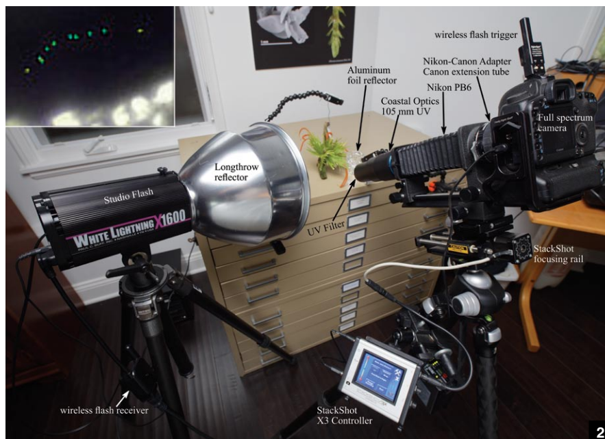
[2] Photographic set-up for UV reflectance z-stacking of orchid flowers. Insert top left: z-stacking artifact from defective pixels. For details see main text.
